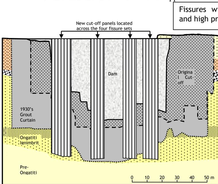
Figure 3: Elevation showing Four Cut-off Panels
