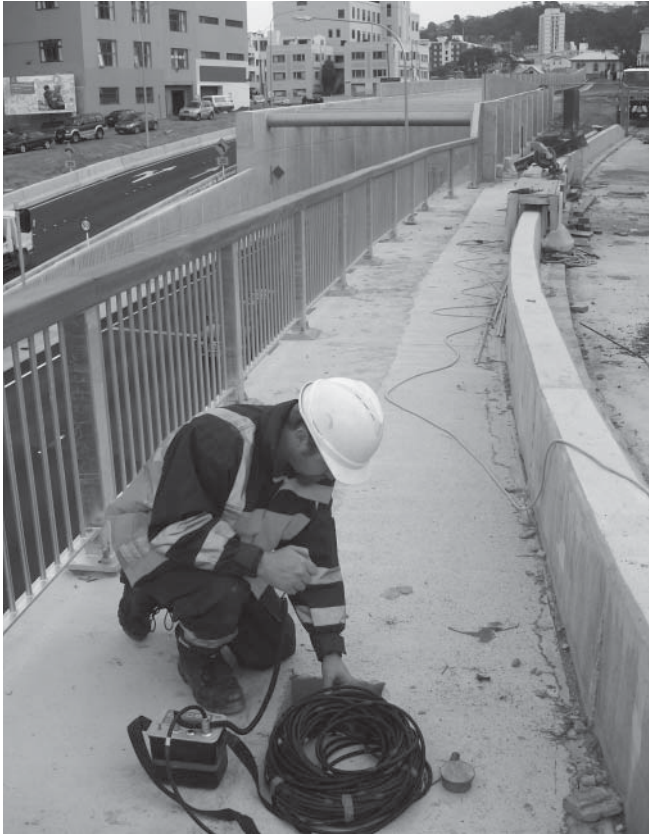
Left: Inclinometer monitoring at the Wellington Inner City Bypass
