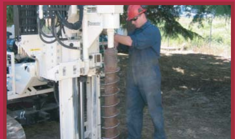
Hollow Stem Auger Soil Coring
