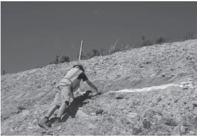
Figure 2: Exposure near crest of highwall in 2005. Geologist is picking at white chalky material whilst standing on highly weathered greywacke rock. Above is pebbly Cape Rodney Formation.
