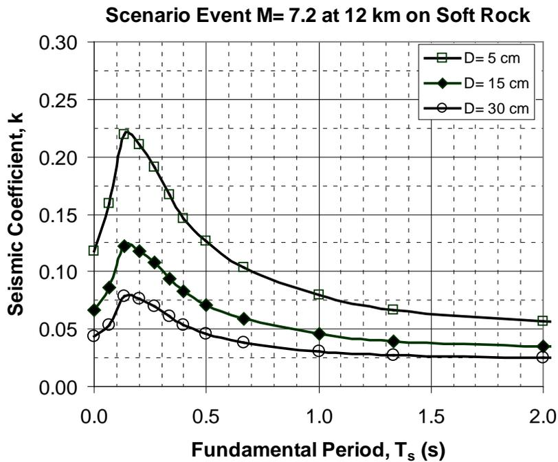
Figure 3. Dependence of the seismic coefficient on the fundamental period of the potential sliding mass for a scenario earthquake (from Bray and Travararou 2009)
