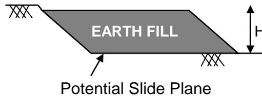
**Figure 4. Illustrative seismic slope stability problem of a compacted earth fill atop a rock site**
