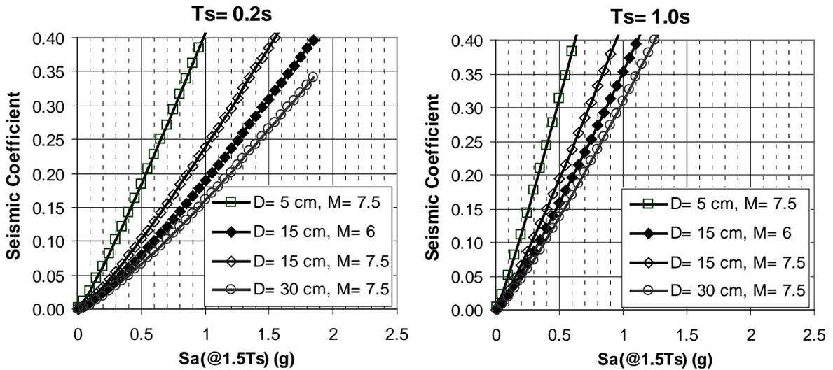
Figure 2. Variation of the seismic coefficient as a function of key seismic slope stability parameters (from Bray and Travararou 2009)
