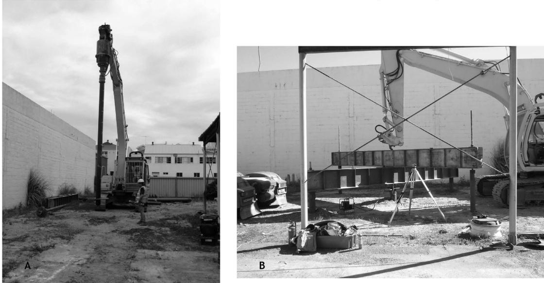
**Figure 1: Full scale pile load test: A-Installation of a test screw pile, B-Pile testing**
