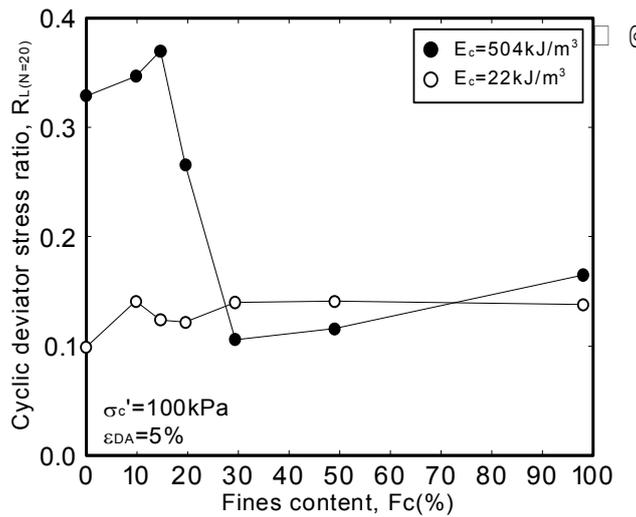
Figure 4: Cyclic shear strength ratio plotted against fines content
