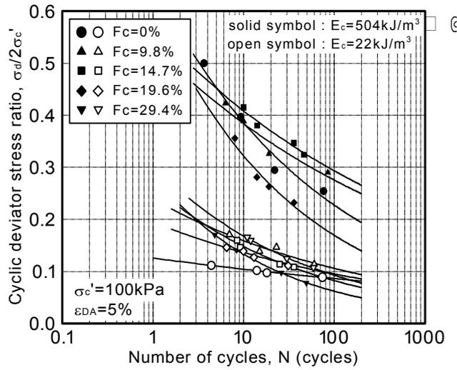
Figure 3: Cyclic shear strength curves
