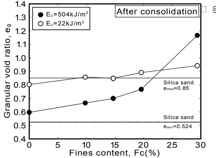
**Figure 2: Relation between granular void ratio and fines content for samples after consolidation**
