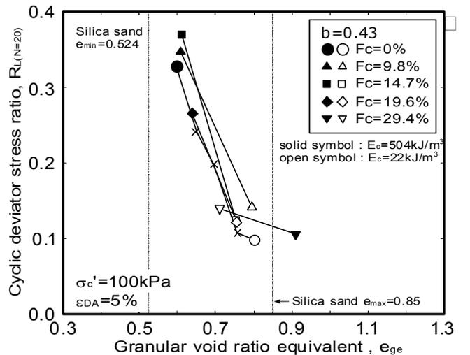
Figure 6: Variation of cyclic shear strength ratio with equivalent granular void ratio
