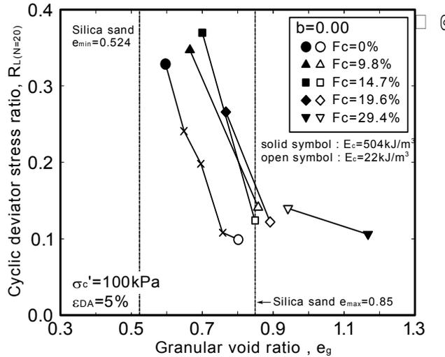
Figure 5: Relation between cyclic shear strength ratio and granular void ratio
