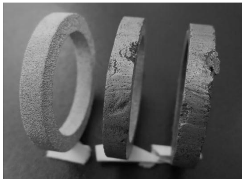
Figure 1: Wear on porous filters. From left to right: a new porous filter, a worn filter which may be reusable at the discretion of the operator and an unusable worn filter.
