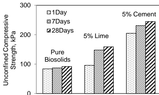
Figure 6. Unconfined Compressive Strength of 1-7-28 days curing samples
