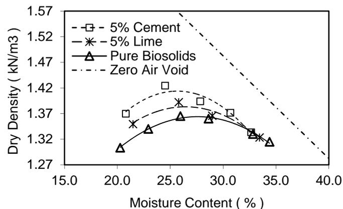
*Figure 4. Compaction curves for pure and stabilised biosolids*
