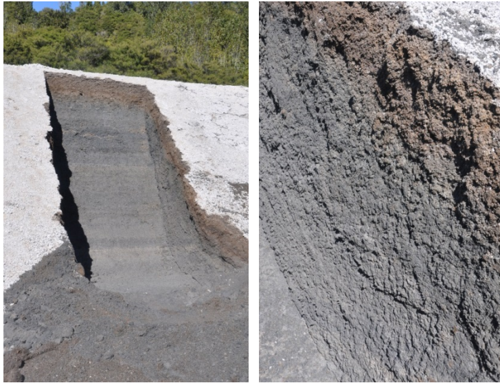
Figure 3. Compacted Primary Solids
