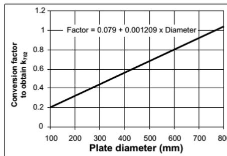
Figure 3: Conversion factor for smaller plate sizes (IAN 73/06, 2009)
