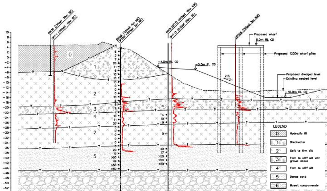
Figure 2: Geotechnical cross section through proposed Oil Berth
