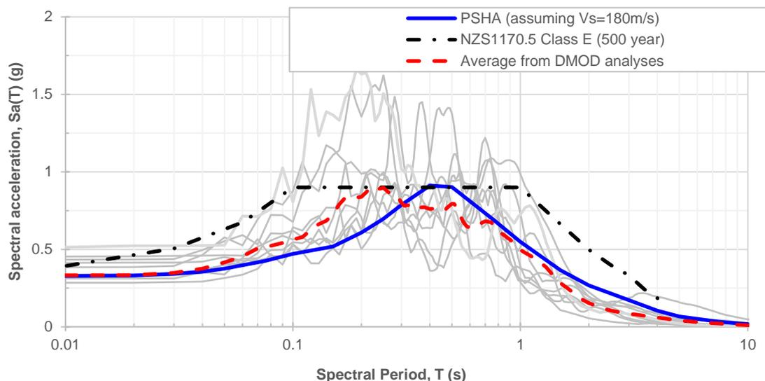
**Figure 3:** Response spectra plot for the CLE event showing the results from the PSHA (blue line), code spectra from NZS1170.5 (black line) and average spectra from the DMOD analyses (red line). The light grey lines are the spectra from individual DMOD analyses.
