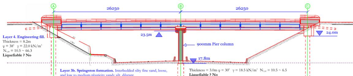
Figure 1: Longitudinal section of the bridge with idealised soil profile
