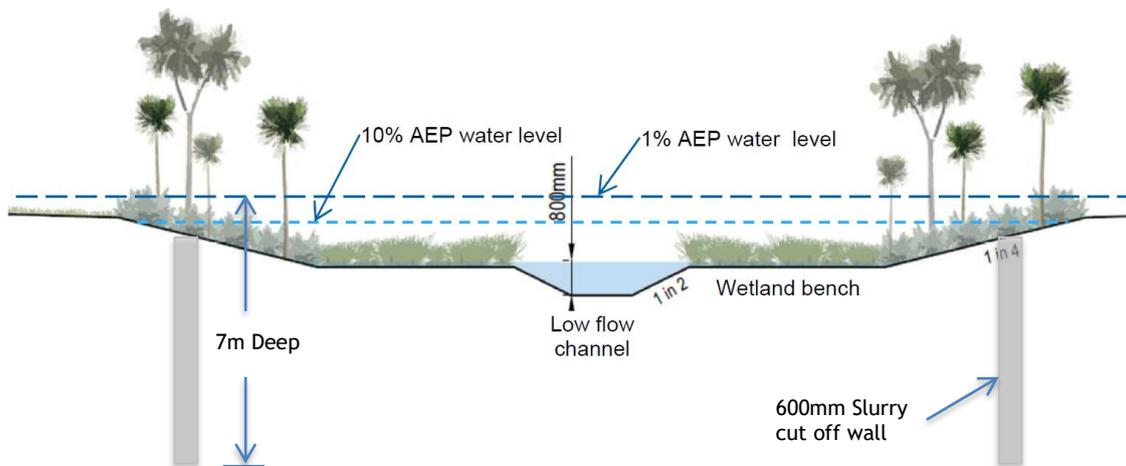
Figure 2: Typical channel section with slurry cut off wall
