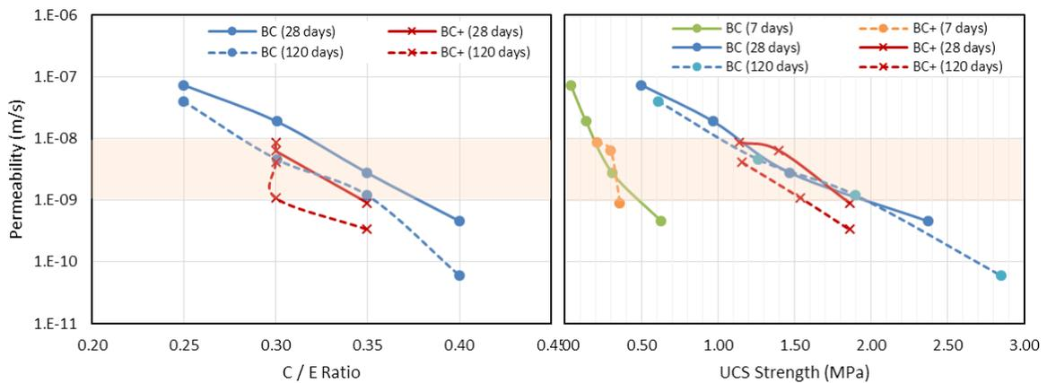
**Figure 4: Laboratory trial summary permeability and strength results**
