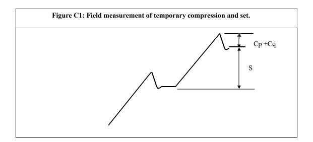
C7.3 If the record card is attached some distance below the pile top, the elastic compression in the upper part of the pile (part of  $C_p$ ) will not be shown on the graph. That compression should be calculated from Table C1 and added to the sum of the temporary compressions used to derive C, i.e.  $C = C_c + C_p + C_q +$  upper pile compression.
