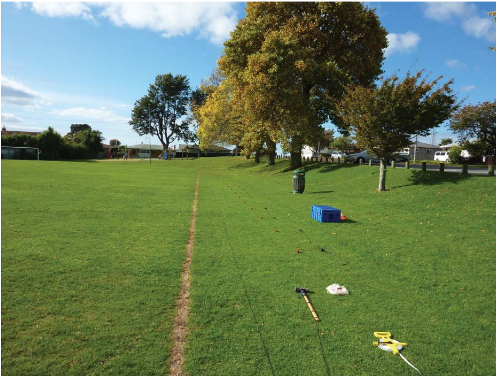
Figure 3: Typical active source test set-up, showing array of geophones, sledgehammer and pad.
