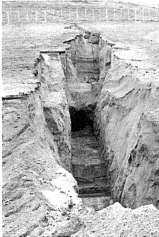
Figure 4. Erosion Tunnel at Drill Pad 64. The Tunnel was Encountered on the Reservoir Side of the Break Out Point
