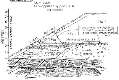
NEAR HORIZONTAL BUT IRREGULAR SURFACE OF FRACTURED IGNIMBRITE ROCK MASS, EXPOSED IN FLOOR OF FAILURE CHANNEL. Logged by W.M.P. 3/2/83
