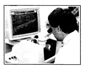
• MPS-2 An analytical micro photogrammetric stereoplotter enabling 3D digitising of structures or topography into AutoCAD, SDR Mapping & Design or Micro Station.
