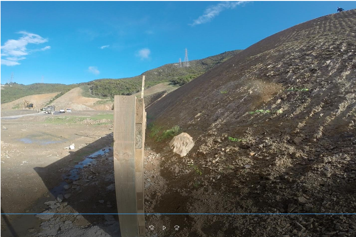
Figure 3: Trial fence, shown just before impact of 54 kg rock that broke some lagging. The researcher who rolled the rock can just be seen top right of picture.
