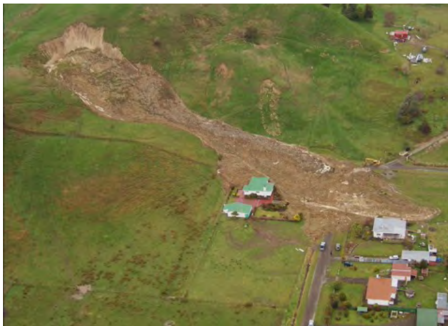
FIGURE 3.14. Earthflow landslide in Hunterville. Note emptying of material at the crown and distance of flow run out downslope.
