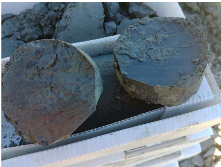
FIGURE 4.7. Landslide shear surface identified by polished surface and striations in core.
