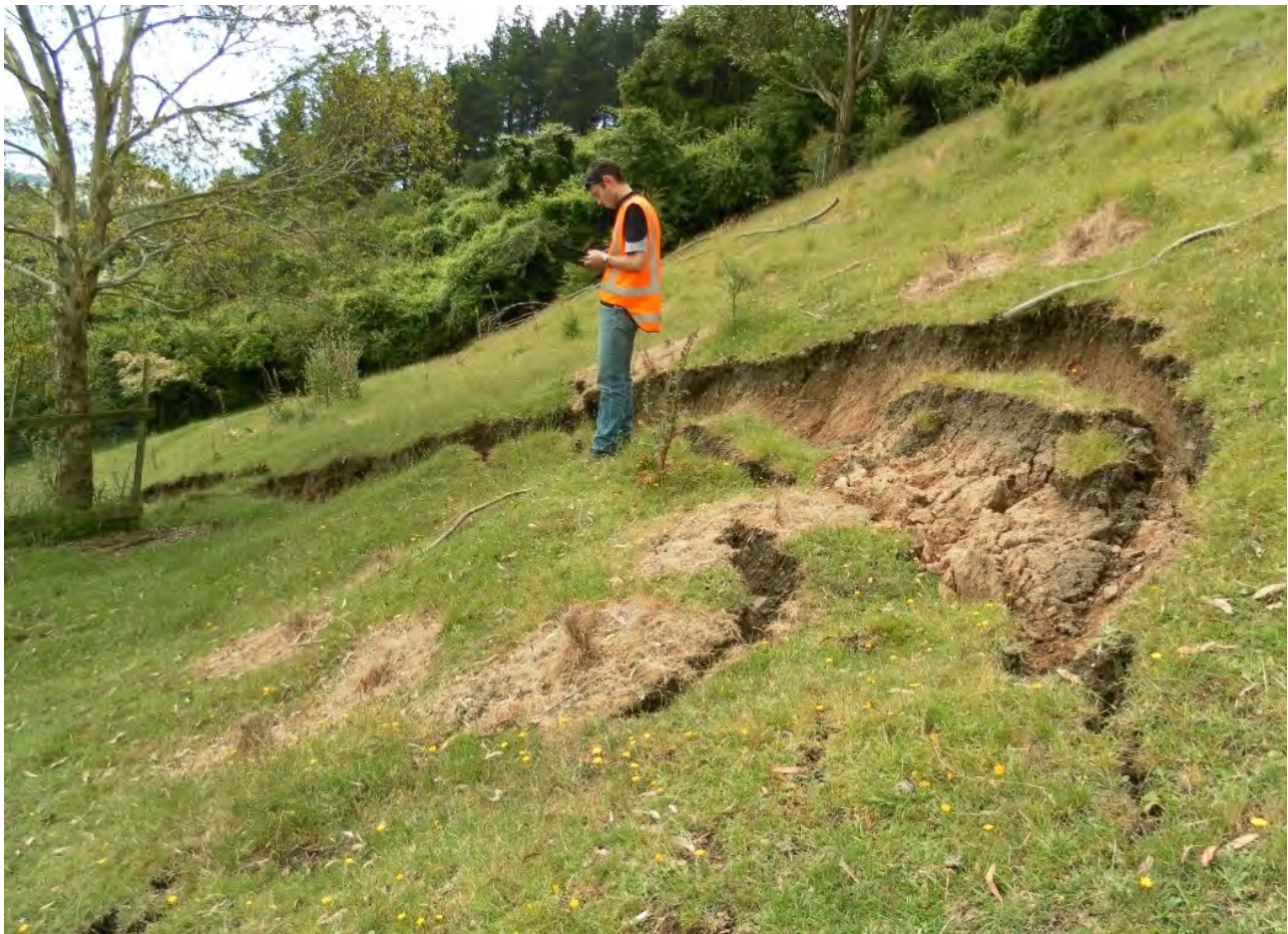
PHOTOGRAPH 3.9. Example of cracking at a landslide head (compare to cracks shown in Figure 3.8)
