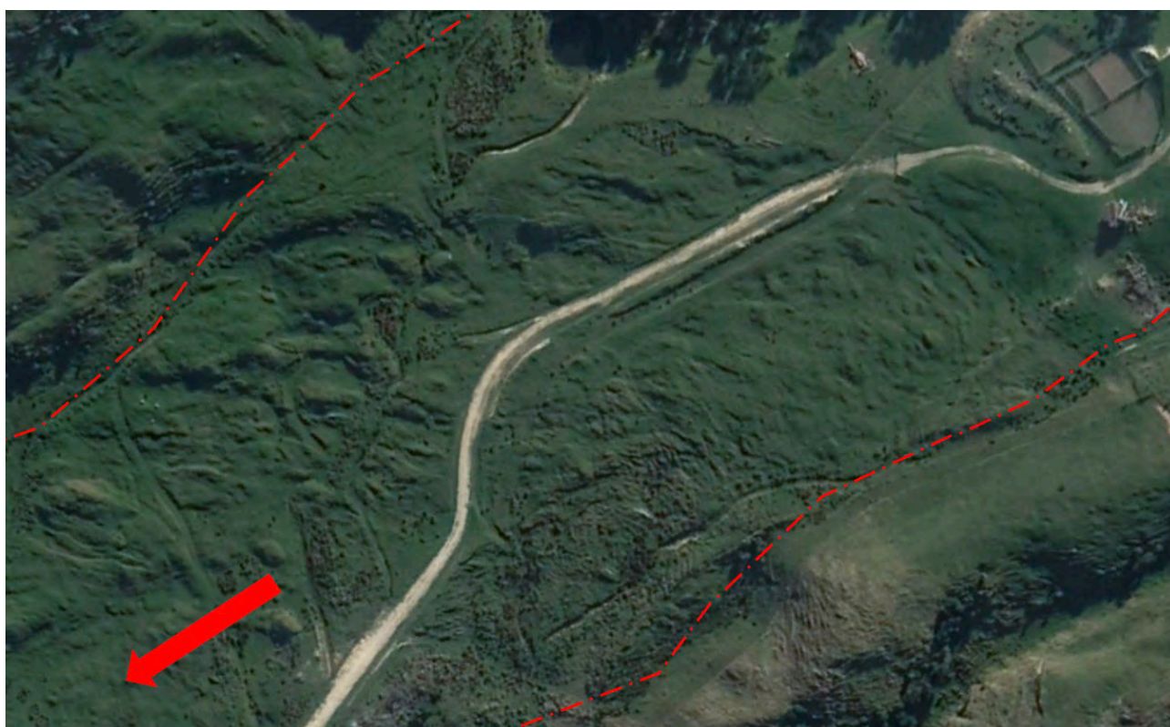
FIGURE 3.1. Hummocky ground on a complex landslide near Pongaroa. Red arrow = direction of movement
