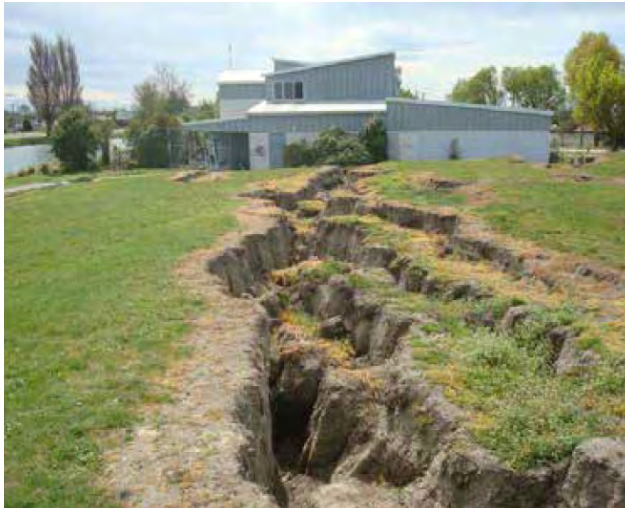
FIGURE 2.8. Lateral Spreading adjacent to the Avon River during the 2010 - 2011 Christchurch Earthquake (Source: Rapid Post Disaster Building Usability Assessment Field Guide)
