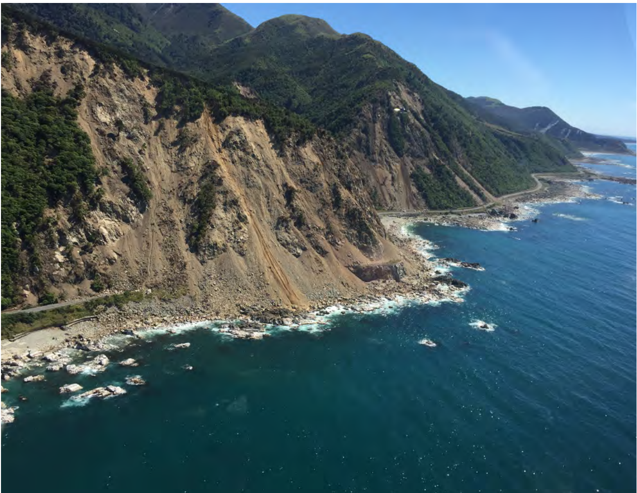
FIGURE 2.4. Debris Avalanche, Kaikoura Coast following the 2018 Earthquake, (Source NCTIR)
