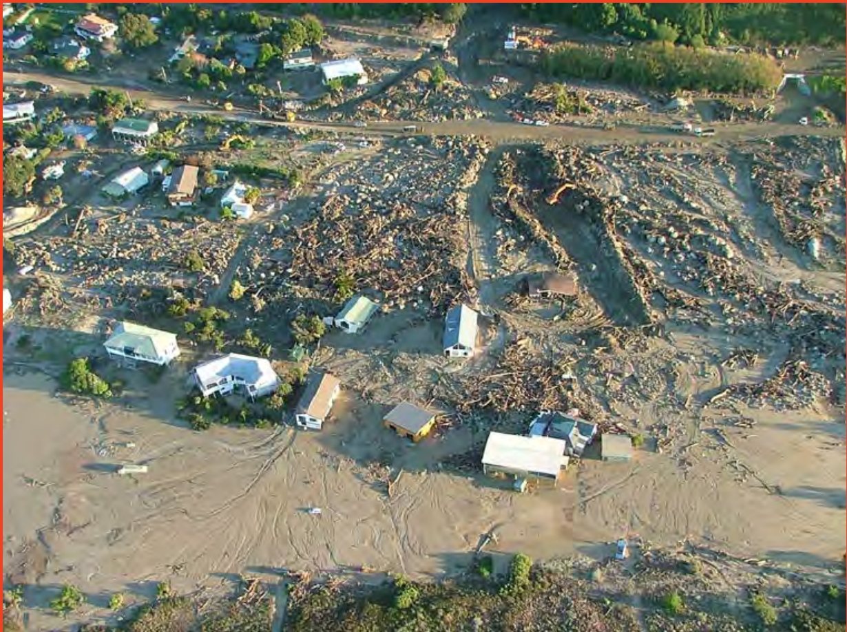
Debris Flow Damage, Awataraki Stream, Matata, following the 18 May 2005 debris flow McSaveney, et al (2005).
