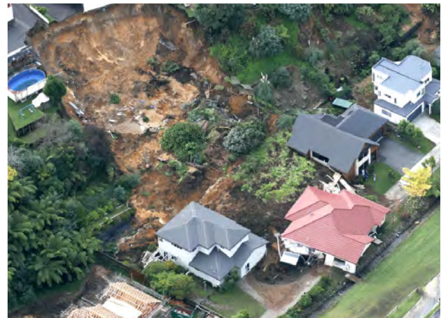
FIGURE 2.6 Rotational Slide, becoming a debris flow downslope
