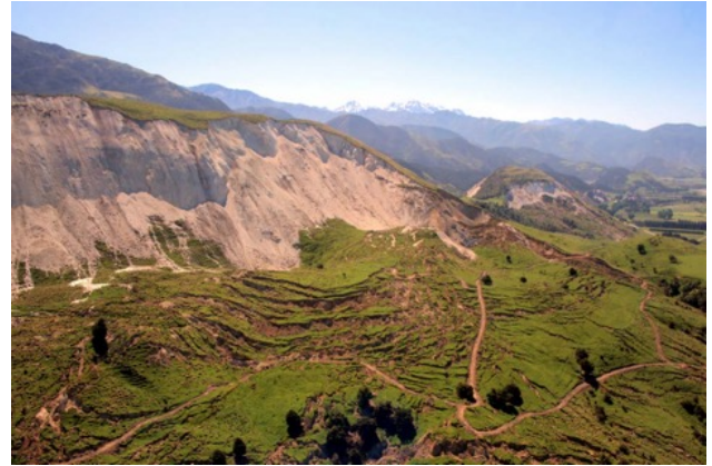
FIGURE 56: Main scarp and upper part of the Sea Front landslide (Jibson et al., 2018).
