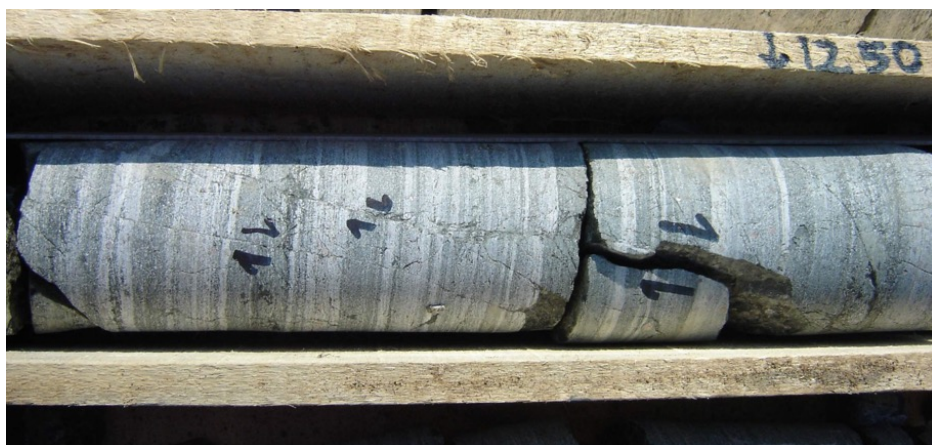
FIGURE 1: (a) Intact rock sample and (b) samples with discontinuities (shears)
