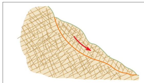
FIGURE 18. Non-planar failure with irregular failure surface in heavily jointed rock mass (Gonzalez & Ferrer, 2011)
