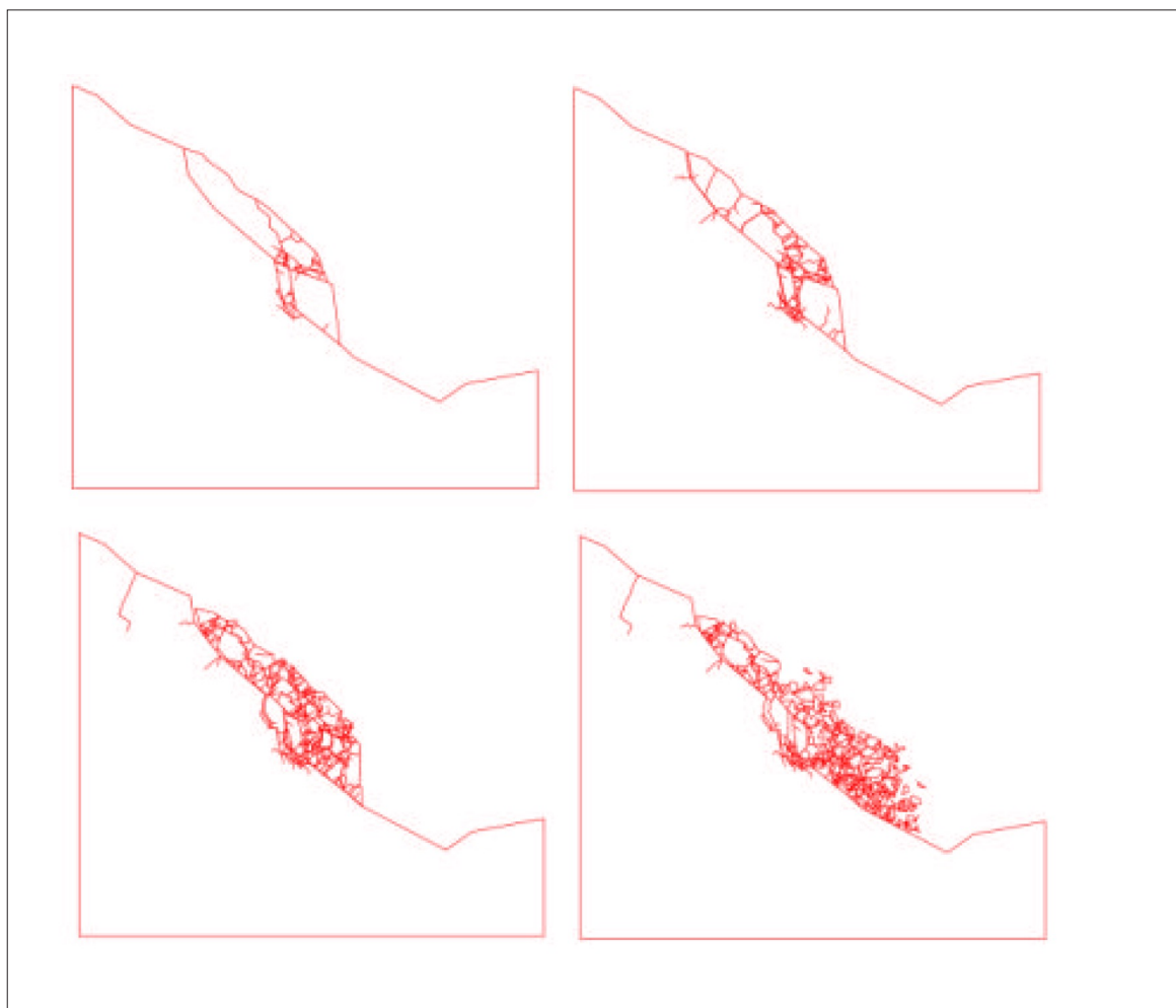
FIGURE 25: Hybrid finite-/distinct element analysis of a rockslide showing several progressive stages of brittle failure (Eberhardt, et al., 2002).
