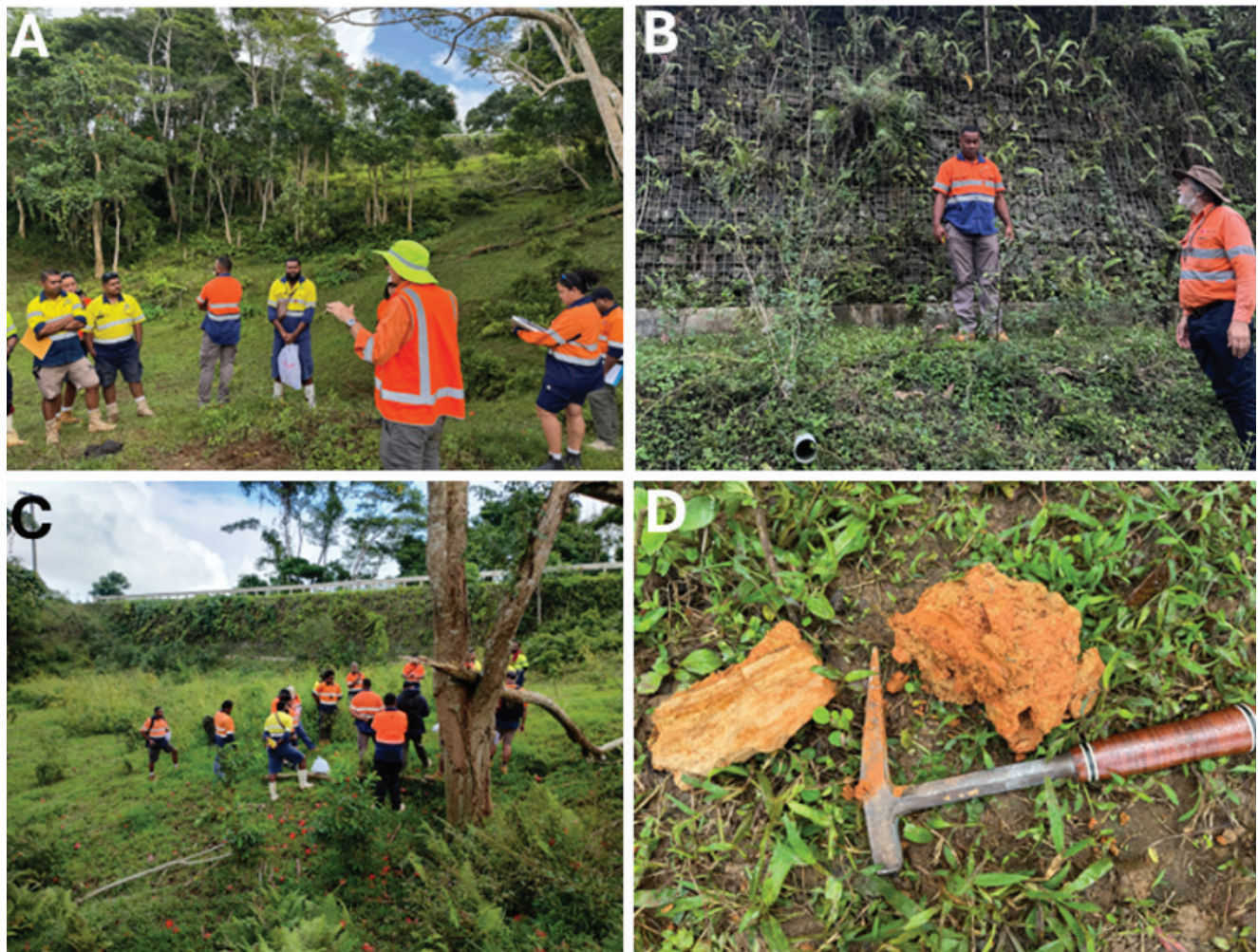
Figure 3: Kasavu Landslide: (A) view upslope from above toe area; (B) gabion wall under re-instated road in headscarp area; (C) break of slope below headscarp; (D) weathered Waidina Sandstone residual materials.
