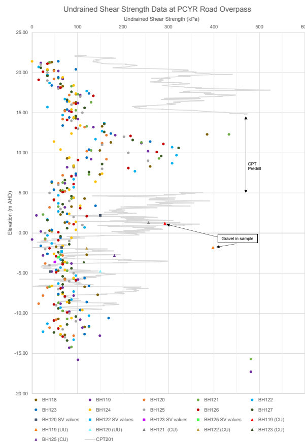
Figure 4: Undrained Shear Strength Data at PCYR Road Overpass
