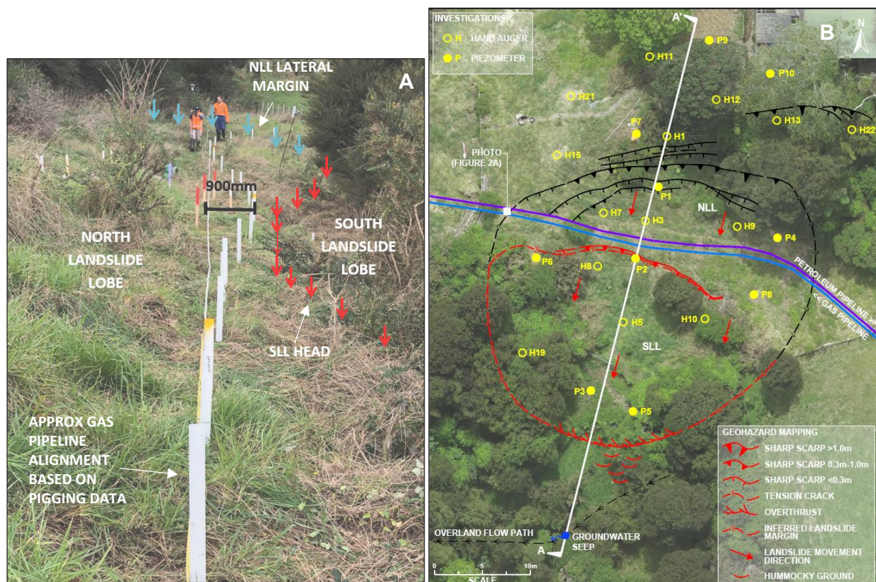
Figure 2: (A) Photo facing east across the landslide showing the inferred downslope deflection from assumed as-built alignment of the gas pipeline. (B) Simplified engineering geology sketch plan. Section A-A' shown on Figure 3.
